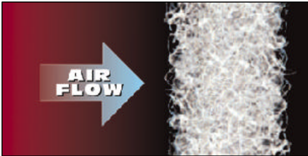
Needling entangles the fibers throughout the entire depth of the media producing high mechanical efficiency.
